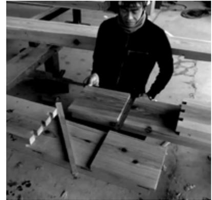
2. Component parts are prefabricated at the carpenter's workshop
