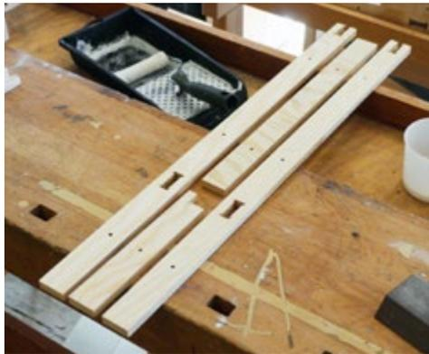
3. Each structural component is laminated from 3 layers
