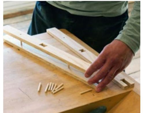
4. CNC-drilled holes and wooden dowels allow us to laminate precisely
