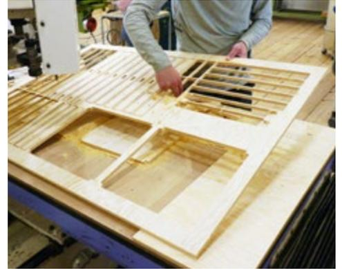
2. All joint parts are cut from 12mm pine plywood
